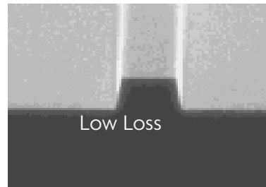
Extremely low loss SiN rib waveguide.
