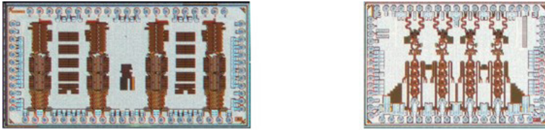
4-channel transimpedance amplifier (left), 4-channel Mach-Zehnder driver (right)
